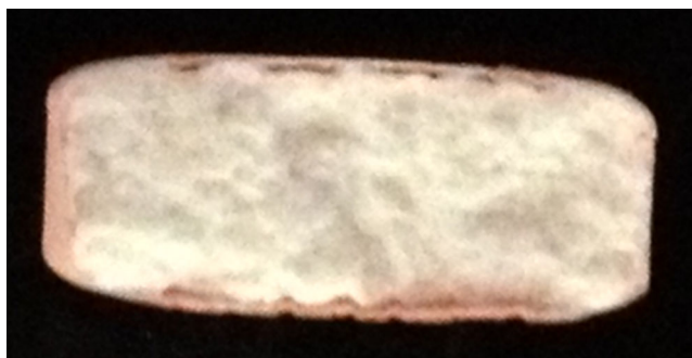
Fig. 9. Cross-section of a coated tablet showing that the underlying cause of logo bridging in this study was the film not adhering well to the tablet substrate
